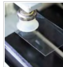
Automated mounting and final coverslip after DAPI
