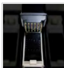
Manual application of oil with an oil stamp for sealing reaction chamber [micro-chamber]
